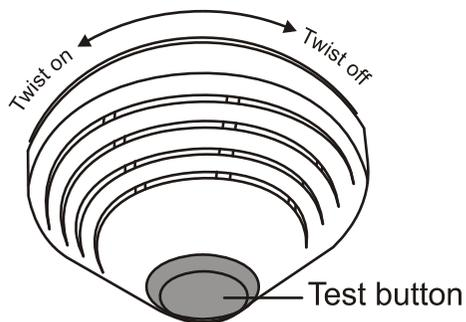
The detector reports fire hazards. It is activated by the presence of smoke or an abnormal temperature increase. Besides sending a report to the system, it also triggers its own siren during an alarm.
