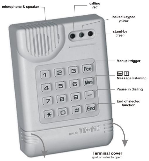
The TD-110 is an automatic dialing device that transmits a prerecorded voice message to 4 telephone numbers to an ordinary or mobile telephone system. It can also send a numeric message to your Pager.
