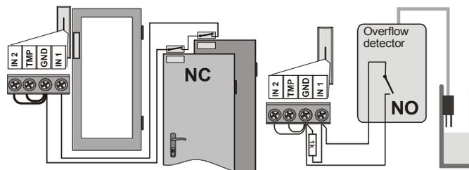
Wiring example for NC ... and NO contacts
